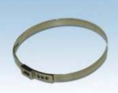
Replacing sleeves requires new clamps to secure sleeves on support tubes. We do not recommend the use of worm-gear-clamps as these clamps may squeeze and crimp the sleeve. This may damage the sleeve or cause air-leakage at the clamp. See our installation instructions for details. V2A clamps (SS304) are stocked, V4A clamps (SS316) are available, too, but non-stock items.
