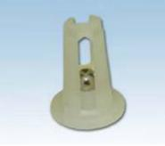
Check valves (non-return-valves) consist of a PP housing containing an 8 mm SS-ball. The stainless-steel ball prevents backflow of sludge into headers in case of damage to the membrane of the disc. Check valves alter the headloss characteristic of JetFlex® disc diffusers, so do not install discs with and without check valve in the same tank or on the same grid. Check valves work best if discs are installed using our clamp adaptors 90N or our rubber saddles, see above.
